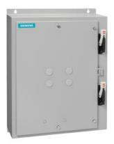
Duplex starter w/o alternator Size 2 Three phase full voltage Solid-state overload relay OLR amp range 13-52A 208VAC 60Hz Coil Combination type Two 60A disconnect switches Enclosure NEMA type 1 Indoor general purpose use
