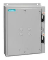
Duplex starter w/o alternator Size 1.75 Three phase full voltage Solid-state overload relay OLR amp range 10-40A 240VAC 50Hz / 277VAC 60Hz Coil Combination type Two 60A disconnect switches Encl NEMA type 4X 304 S. Steel Water/dust tight non-corrosive
