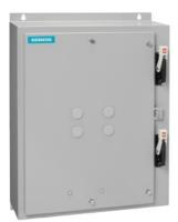
Duplex starter w/o alternator, Size 1 3/4, Three phase full voltage, Solid-state overload relay, OLR amp range 10-40A, 380-440/440-480V 50/60Hz coil, Combination type, Two 40A circuit breakers, Enc NEMA type 4 painted steel, Water/dust tight for outdoors
