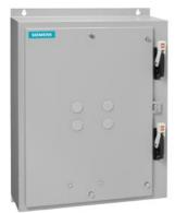
Duplex starter w/o alternator Size 1.75 Three phase full voltage Solid-state overload relay OLR amp range 10-40A 24VAC 50-60Hz Coil Combination type Two 60A disconnect switches Encl NEMA type 4 painted steel Water/dust tight weather proof
