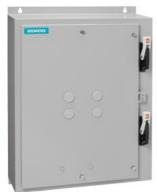
Duplex starter w/o alternator Size 1 Three phase full voltage Solid-state overload relay OLR amp range 10-40A 110VAC 50Hz / 120VAC 60Hz Coil Combination type Two 30A disconnect switches Enclosure NEMA type 1 Indoor general purpose use
