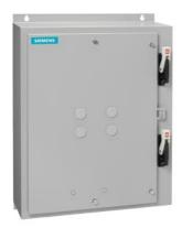
Duplex starter w/o alternator, Size 1, Three phase full voltage, Solid-state overload relay, OLR amp range 5.5-22A, 24VAC 50-60Hz coil, Combination type, Two 25A circuit breakers, Enc NEMA type 4 painted steel, Water/dust tight for outdoors
