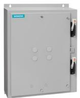
Duplex starter w/o alternator Size 1 Three phase full voltage Solid-state overload relay OLR amp range 3-12A 208VAC 60Hz Coil Combination type Two 30A disconnect switches Encl NEMA type 4 painted steel Water/dust tight weather proof
