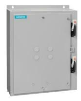
Duplex starter w/o alternator Size 1 Three phase full voltage Solid-state overload relay OLR amp range 3-12A 24VAC 50-60Hz Coil Combination type Two 30A disconnect switches Enclosure NEMA type 1 Indoor general purpose use
