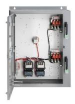
Duplex starter with alternator Size 1 Three phase full voltage Solid-state overload relay OLR amp range 3-12A 110VAC 50Hz / 120VAC 60Hz Coil Combination type Two 30A disconnect switches Encl NEMA type 4 painted steel Water/dust tight weather proof
