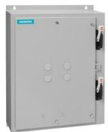
Duplex starter w/o alternator Size 1 Three phase full voltage Solid-state overload relay OLR amp range 0.75-3.4A 240VAC 50Hz / 277VAC 60Hz Coil Combination type Two 30A disconnect switches Enclosure NEMA type 1 Indoor general purpose use
