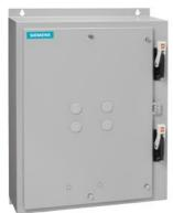
Duplex starter w/o alternator Size 1 Three phase full voltage Solid-state overload relay OLR amp range 0.75-3.4A 110VAC 50Hz / 120VAC 60Hz Coil Combination type Two 30A disconnect switches Enclosure NEMA type 1 Indoor general purpose use
