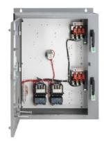
Duplex starter with alternator Size 1 Three phase full voltage Solid-state overload relay OLR amp range 0.75-3.4A 110VAC 50Hz / 120VAC 60Hz Coil Combination type Two 30A disconnect switches Encl NEMA type 4X 304 S. Steel Water/dust tight non-corrosive
