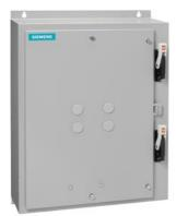
Duplex starter w/o alternator Size 1 Three phase full voltage Solid-state overload relay OLR amp range 0.25-1A 240VAC 50Hz / 277VAC 60Hz Coil Combination type Two 30A disconnect switches Encl NEMA type 4 painted steel Water/dust tight weather proof
