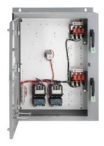
Duplex starter with alternator Size 1 Three phase full voltage Solid-state overload relay OLR amp range 0.25-1A 110VAC 50Hz / 120VAC 60Hz Coil Combination type Two 30A disconnect switches Enclosure NEMA type 1 Indoor general purpose use
