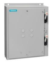
Duplex starter w/ alternator, Size 0, Three phase full voltage, Solid-state overload relay, OLR amp range 5.5-22A, 110V 50Hz / 120V 60Hz coil, Combination type, Two 25A circuit breakers, Encl NEMA type 4X 304 S-Steel, Water/dust tight noncorrosive
