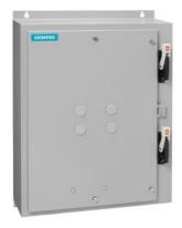
Duplex starter w/o alternator Size 0 Three phase full voltage Solid-state overload relay OLR amp range 3-12A 110VAC 50Hz / 120VAC 60Hz Coil Combination type Two 30A disconnect switches Encl NEMA type 4 painted steel Water/dust tight weather proof
