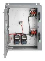
Duplex starter with alternator Size 0 Three phase full voltage Solid-state overload relay OLR amp range 0.75-3.4A 110VAC 50Hz / 120VAC 60Hz Coil Combination type Two 30A disconnect switches Encl NEMA type 4X 304 S. Steel Water/dust tight non-corrosive
