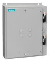
Duplex starter w/o alternator, Size 0, Three phase full voltage, Solid-state overload relay, OLR amp range 0.25-1A, 240V 50Hz / 277V 60Hz coil, Combination type, Two 3A circuit breakers, Enc NEMA type 4 painted steel, Water/dust tight for outdoors
