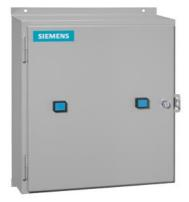
Duplex starter w/o alternator, Size 3, Three phase full voltage, Solid-state overload relay, OLR amp range 25-100A, 190-220/220-240V 50/60Hz coil, Non-combination type, Encl NEMA type 4X 304 S-Steel, Water/dust tight noncorrosive
