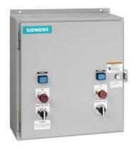
Duplex starter w/ alternator, Size 3, Three phase full voltage, Solid-state overload relay, OLR amp range 25-100A, 110V 50Hz / 120V 60Hz coil, Non-combination type, Enclosure NEMA type 12, Dust/drip proof for indoors
