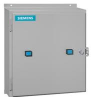
Duplex starter w/o alternator, Size 2 1/2, Three phase full voltage, Solid-state overload relay, OLR amp range 25-100A, 380-440/440-480V 50/60Hz coil, Non-combination type, Encl NEMA type 4X 304 S-Steel, Water/dust tight noncorrosive
