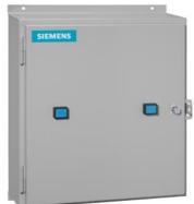
Duplex starter w/o alternator, Size 2, Three phase full voltage, Solid-state overload relay, OLR amp range 13-52A, 24VAC 50-60Hz coil, Non-combination type, Enc NEMA type 4 painted steel, Water/dust tight for outdoors
