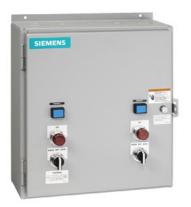
Duplex starter w/ alternator, Size 1 3/4, Three phase full voltage, Solid-state overload relay, OLR amp range 10-40A, 110V 50Hz / 120V 60Hz coil, Noncombination type, Enclosure NEMA type 12, Dust/drip proof for indoors
