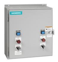
Duplex starter w/ alternator, Size 1, Three phase full voltage, Solid-state overload relay, OLR amp range 5.5-22A, 110V 50Hz / 120V 60Hz coil, Non-combination type, Enclosure NEMA type 12, Dust/drip proof for indoors
