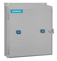
Duplex starter w/o alternator, Size 1, Three phase full voltage, Solid-state overload relay, OLR amp range 3-12A, 380-440/440-480V 50/60Hz coil, Non-combination type, Enclosure NEMA type 12, Dust/drip proof for indoors
