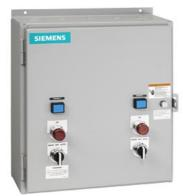
Duplex starter w/ alternator, Size 1, Three phase full voltage, Solid-state overload relay, OLR amp range 3-12A, 110V 50Hz / 120V 60Hz coil, Non-combination type, Encl NEMA type 4X 304 S-Steel, Water/dust tight noncorrosive
