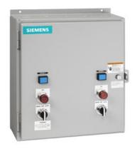
Duplex starter w/ alternator, Size 0, Three phase full voltage, Solid-state overload relay, OLR amp range 3-12A, 110V 50Hz / 120V 60Hz coil, Non-combination type, Enc NEMA type 4 painted steel, Water/dust tight for outdoors
