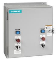
Duplex starter w/ alternator, Size 0, Three phase full voltage, Solid-state overload relay, OLR amp range 0.75-3.4A, 110V 50Hz / 120V 60Hz coil, Non-combination type, Enclosure NEMA type 12, Dust/drip proof for indoors
