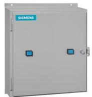
Duplex starter w/o alternator, Size 0, Three phase full voltage, Solid-state overload relay, OLR amp range 0.25-1A, 380-440/440-480V 50/60Hz coil, Non-combination type, Enc NEMA type 4 painted steel, Water/dust tight for outdoors
