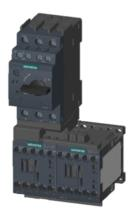
Fuseless motor starter Reversing operation 600VAC Size S00 3.5-5A 24V DC screw connection For screw mounting Or 35 mm rail-mounting Type of coordination 1 1NO+1NC (MSP) 1NC (per contactor)
