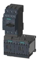
Fuseless motor starter Reversing operation 600VAC Size S00 0.7-1A 24V DC screw connection For screw mounting Or 35 mm rail-mounting Type of coordination 2 IQ = 150 KA Also full fills type Of coordination 1 1NO+1NC (MSP) 1NC (per contactor)
