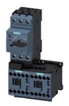
Load feeder fuseless, Reversing duty 400 V AC, Size S00 1.80...2.50 A 230 V AC screw terminal for installation on standard mounting rail (also fulfills type of coordination 1) Type of coordination 2, Iq = 150 kA 1 NC (contactor)
