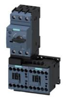
Load feeder fuseless, Reversing duty 400 V AC, Size S00 0.28...0.40 A 24 V DC screw terminal for installation on standard mounting rail (also fulfills type of coordination 1) Type of coordination 2, Iq = 150 kA 1 NC (contactor)
