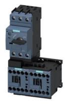
Load feeder fuseless, Reversing duty 400 V AC, Size S00 0.28...0.40 A 230 V AC screw terminal for installation on standard mounting rail (also fulfills type of coordination 1) Type of coordination 2, Iq = 150 kA 1 NC (contactor)
