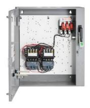
2-speed 3-phase motor starter Size 1 One winding consequent pole Constant or variable torque Solid-state overload relays Low SPD OLR range 3-12A High SPD OLR range 3-12A 110V 50HZ / 120V 60HZ coil Combination type 30Amp disconnect switch Enclosure NEMA type 4/12 Water/dust tight for outdoors
