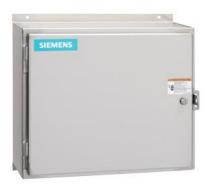
2-speed 3-phase motor starter Size 1 Two separate windings Constant horsepower Solid-state overload relays Low SPD OLR range 3-12A High SPD OLR range 5.5-22A 110V 50HZ / 120V 60HZ coil Enclosure NEMA type 12 Dust/drip proof for indoors
