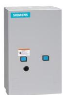
2-speed 3-phase motor starter, Size 1, Two separate windings, Constant or variable torque, Solid-state overload relays, Low Spd OLR range 0.75-3.4A, High Spd OLR range 0.75-3.4A, 24VAC 50-60Hz coil, Enclosure NEMA type 1, Indoor general purpose use
