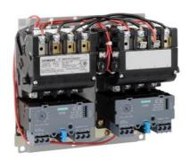
2-speed 3-phase motor starter Size 1 Two separate windings Constant or variable torque Solid-state overload relays Low SPD OLR range 0.25-1A High SPD OLR range 0.75-3.4A 110V 50HZ / 120V 60HZ coil Enclosure NEMA type (open) No enclosure
