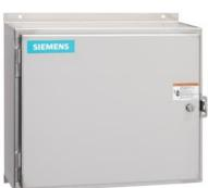
2-speed 3-phase motor starter, Size 0, Two separate windings, Constant or variable torque, Solid-state overload relays, Low Spd OLR range 3-12A, High Spd OLR range 3-12A, 110V 50Hz / 120V 60Hz coil, Encl NEMA type 4X 304 S-Steel, Water/dust tight noncorrosive
