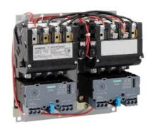
2-speed 3-phase motor starter Size 0 Two separate windings Constant or variable torque Solid-state overload relays Low SPD OLR range 3-12A High SPD OLR range 3-12A 110-120/220-240VAC 60HZ coil Enclosure NEMA type (open) No enclosure
