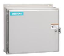
2-speed 3-phase motor starter Size 0 Two separate windings Constant horsepower Solid-state overload relays Low SPD OLR range 3-12A High SPD OLR range 3-12A 24VAC 50-60HZ coil Enclosure NEMA type 12 Dust/drip proof for indoors
