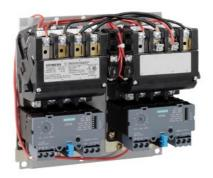
2-speed 3-phase motor starter Size 0 One winding consequent pole Constant or variable torque Solid-state overload relays Low SPD OLR range 0.75-3.4A High SPD OLR range 3-12A 380-440/440-480V 50/60HZ coil Enclosure NEMA type (open) No enclosure
