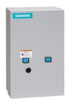
2-speed 3-phase motor starter, Size 0, Two separate windings, Constant or variable torque, Solid-state overload relays, Low Spd OLR range 0.75-3.4A, High Spd OLR range 0.75-3.4A, 24VAC 50-60Hz coil, Enclosure NEMA type 1, Indoor general purpose use
