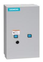
2-speed 3-phase motor starter, Size 0, Two separate windings, Constant horsepower, Solid-state overload relays, Low Spd OLR range 0.75-3.4A, High Spd OLR range 0.75-3.4A, 110V 50Hz / 120V 60Hz coil, Enclosure NEMA type 1, Indoor general purpose use
