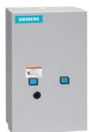
2-speed 3-phase motor starter, Size 0, Two separate windings, Constant or variable torque, Solid-state overload relays, Low spd OLR range 0.25-1A, High Spd OLR range 0.75-3.4A, 110V 50Hz / 120V 60Hz coil, Enclosure NEMA type 1, Indoor general purpose use
