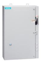
Reversing motor starter, Size 1 3/4, Three phase full voltage, Solid-state overload relay, OLR amp range 10-40A, Combination type, 40A circuit breaker, Enclosure NEMA type 4/12, Water/dust tight for outdoors
