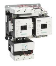
Reversing motor starter Size 5 Three phase full voltage Solid-state overload relay OLRelay amp range 55-250A 23-26V 50-60HZ/DC coil Non-combination type Enclosure type (open)
