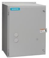
Reversing motor starter, Size 4, Three phase full voltage, Solid-state overload relay, OLR amp range 50-200A, Non-combination type, Enclosure type 12, Dust/drip proof for indoors, Standard width enclosure
