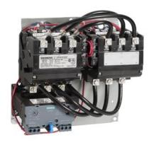
Reversing motor starter Size 3 Three phase full voltage Solid-state overload relay OLRelay amp range 25-100A 24VAC 50-60HZ coil Non-combination type Enclosure type (open)
