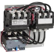
Reversing motor starter Size 3 Three phase full voltage Solid-state overload relay OLRelay amp range 25-100A 110-120/220-240VAC 60HZ coil Non-combination type Enclosure type (open)
